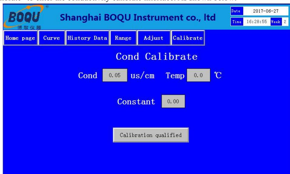
After entering the calibration interface, the conductivity electrode is taken out and placed vertically in 1413us/cm standard solution. After the measured value is stable, the calibration is completed according to the calibration.
