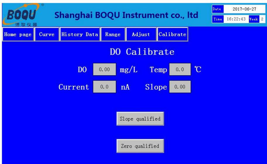
After entering the calibration interface, the dissolved oxygen electrode is taken out and placed vertically in saturated oxygen or air. After the current value is stable, the calibration is completed according to the slope. Under normal circumstances, do not need to zero calibration. For calibration, then the electrode placed in oxygen-free water, according to zero qualified to complete zero calibration.
