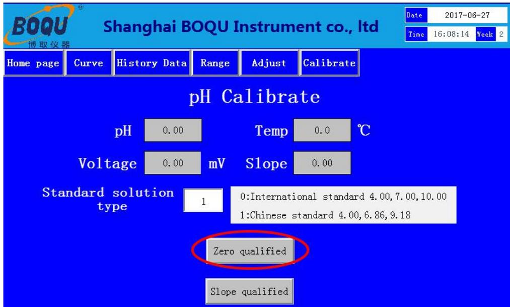
Then put the pH electrode into 4.00 or 9.18 standard, when the data stable, click “Slope qualified” key
