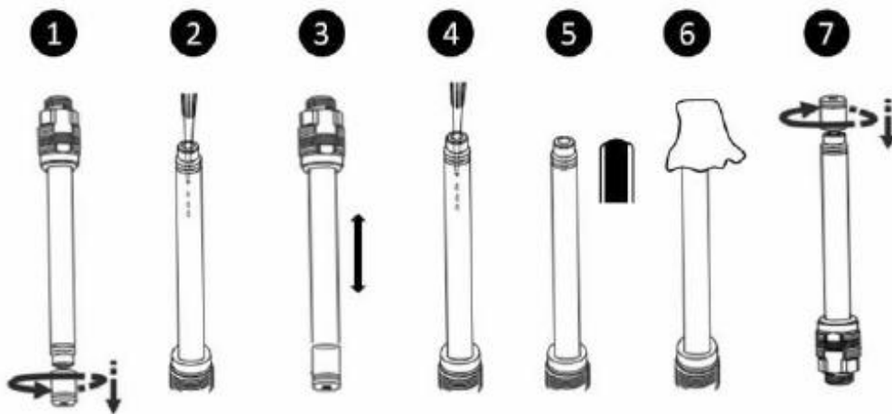
Figure 19 Diagram of Replacing Electrolyte
