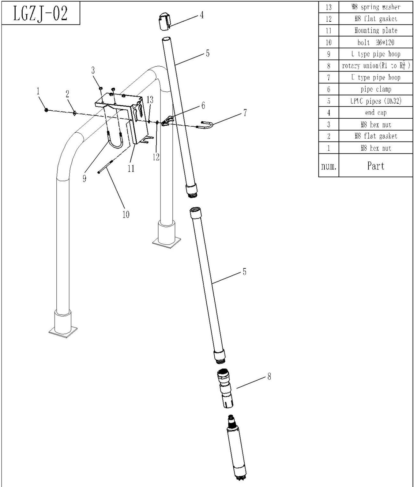
Figure 8 Railing fixed installation sketch map
