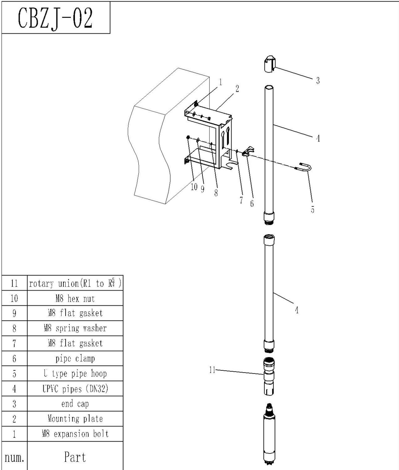
Figure 6 Quick Dismantling pool side installation sketch map
