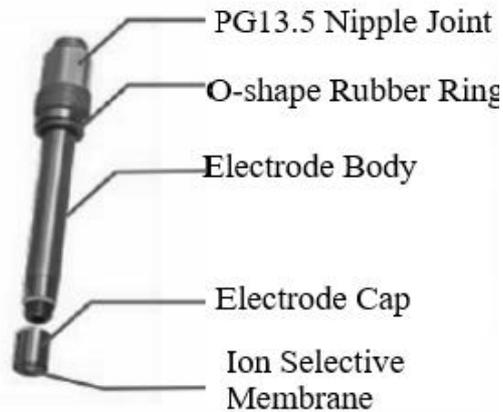
Figure 9 Diagram of Ammonia Nitrogen Electrode
