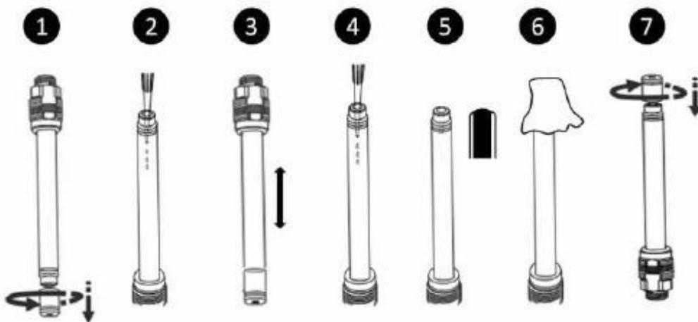
Figure 10 Diagram of Replacing Electrolyte
